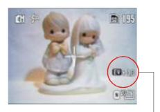
After you manually set the exposure value in — "Manual" capture mode, the exposure value will be shown on the LCD screen.
